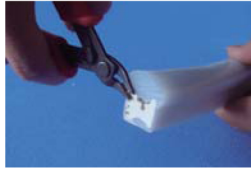
b. Cut out the rest Conductors
